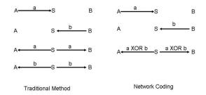
Figure.1 Network Coding versus Traditional Method of Communication.
